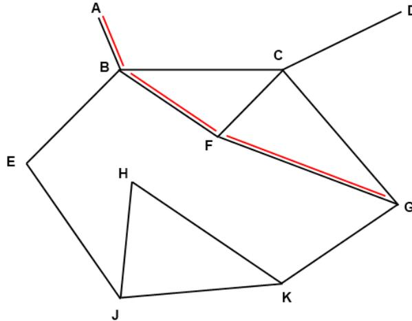
Inner nodes on the path A-B-F-G are B and F. B has 4 edges, F has 3, so the distance is 7. The path A-B-C-G has a distance value of 8, since B has 4 edges and C as well.
