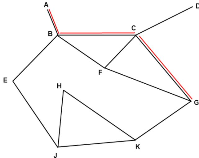
In this case, a shortest path from A to G is A-B-C-G, and the distance is 3, since three edges are involved. As can be seen, this definition doesn't yield a unique path. A-B-F-G would also be possible.
